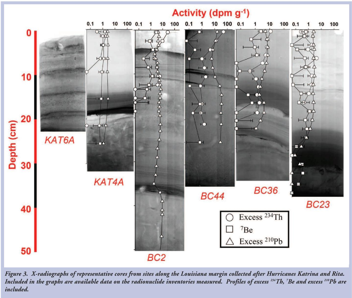
Figure 3. X-radiographs of representative cores from sites along the Louisiana margin collected after Hurricanes Katrina and Rita. Included in the graphs are available data on the radionuclide inventories measured. Profiles of excess <sup>234</sup>Th, <sup>7</sup>Be and excess <sup>210</sup>Pb are included.
