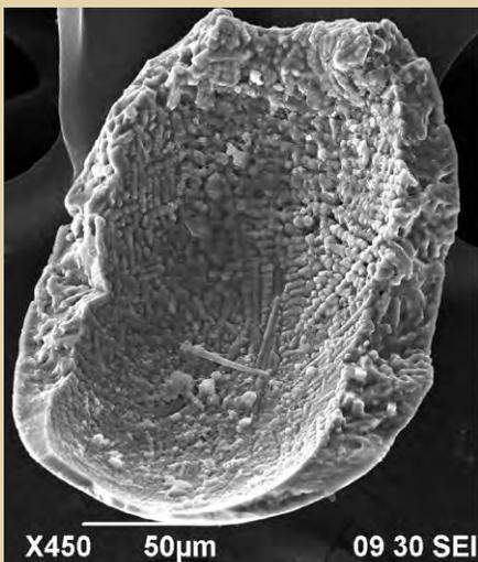
Figure 11. Dendritic structure of a broken iron bead.
