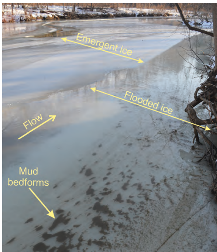
Cover image: Overview of the ice flume looking downstream. The flooded portion of the ice varied between 3-4 m wide and was up to ~10 cm deep.
