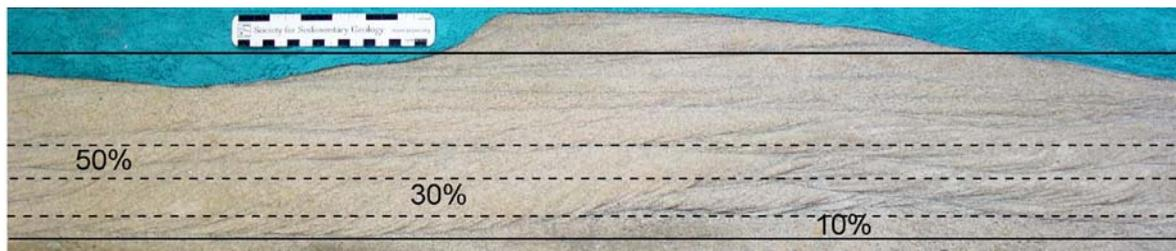
**Figure S3.** Methodological approach for testing the Leclair-Bridge model. Upper and lower lines define the average deposit thickness. Dashed lines are reference datum for measuring cross-set thickness of deposits representing only 50%, 30%, and 10% of the original deposit.
