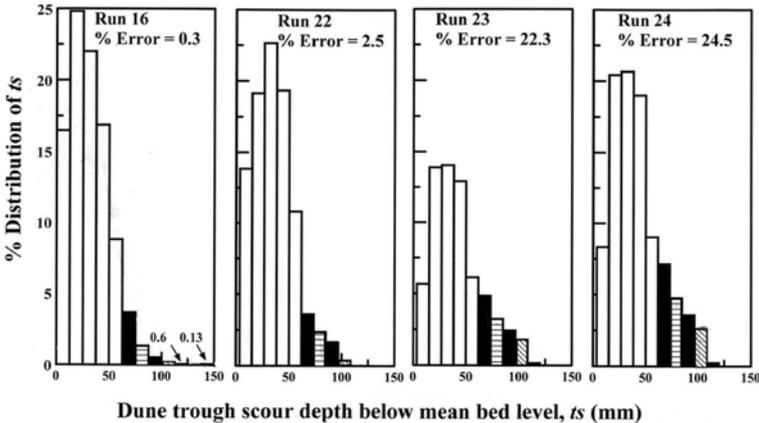
**Figure S4.** Relative distributions of trough scour depth below mean bed level,  $t_s$ , of individual dunes.
