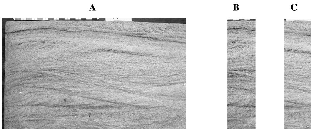
**Figure S6.** Experimental deposit showing cross-set boundaries due to dune climbing as seen A) in a 2D view, or B) and C) in cores. Scale is in centimetres (see video S4; more examples can be found on Picture files S1A-E). Video S1 is from Run 12; distance between flume sections (dark frame) is 1.5 m.
