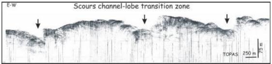
Fig. 1.- TOPAS seismic profile showing the scours identified immediately downslope the Cap Ferret channel mouth.
