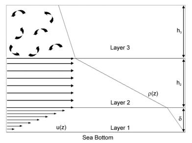
Fig.1. Three layer model for turbidity current where  $\Box \ll h2$ , h3. The stick diagram of the velocity profile u(z) and the density profile  $\Box(z)$  are shown.
