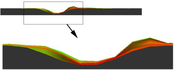
Vertical cross-section view of channel deposits at the exit of a meander bend. Sandy deposits are coded in red going through to green for fine clay deposits. The channel is about 600m wide and 25 meters deep.
